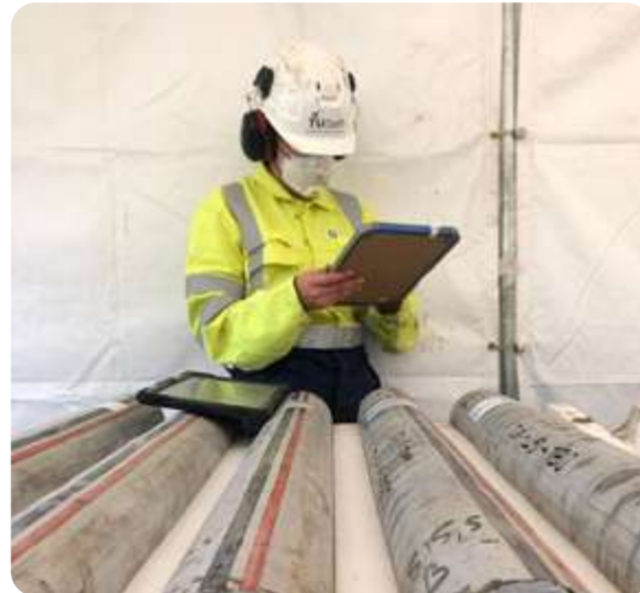
Core description on the drill site. Core barrels were cut in 1 m segments and transported to the core storage on TUD campus.
