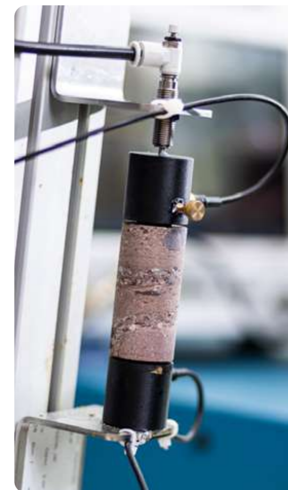
Lab set up with a Rotliegend rock plug to measure the acoustic wave velocity.
