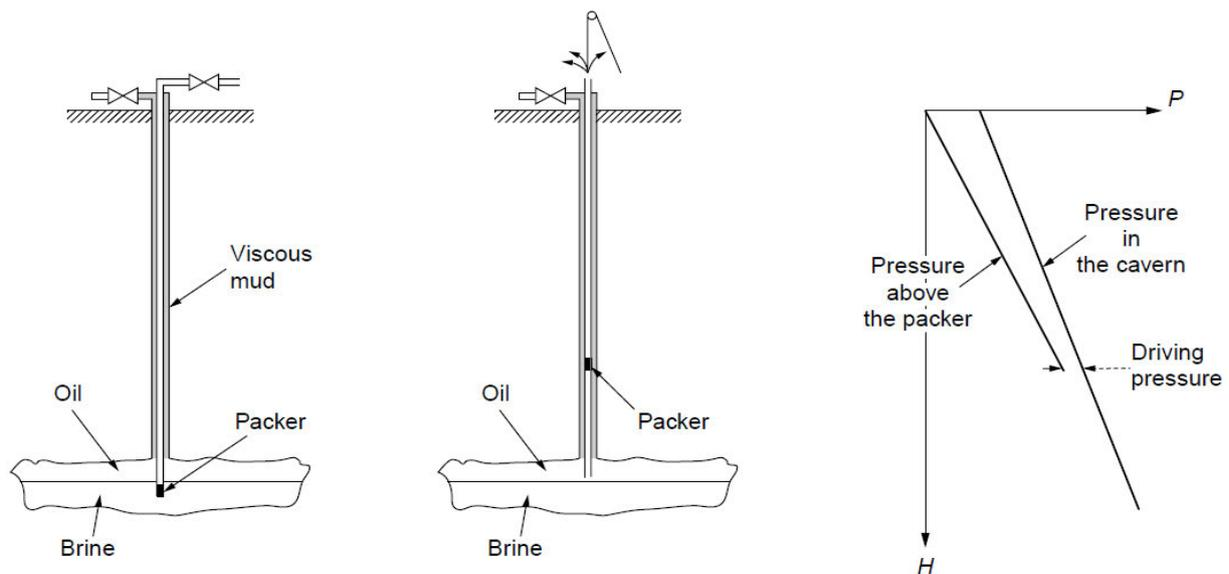
Figure 19 Schematic of the West Hackberry blow out. Showing the rise of the inflatable packer on the left and middle figure. The figure on the right shows the increasing pressure differential between the pressure above the packer and the pressure in the cavern. From Bérest & Brouard (2003).
