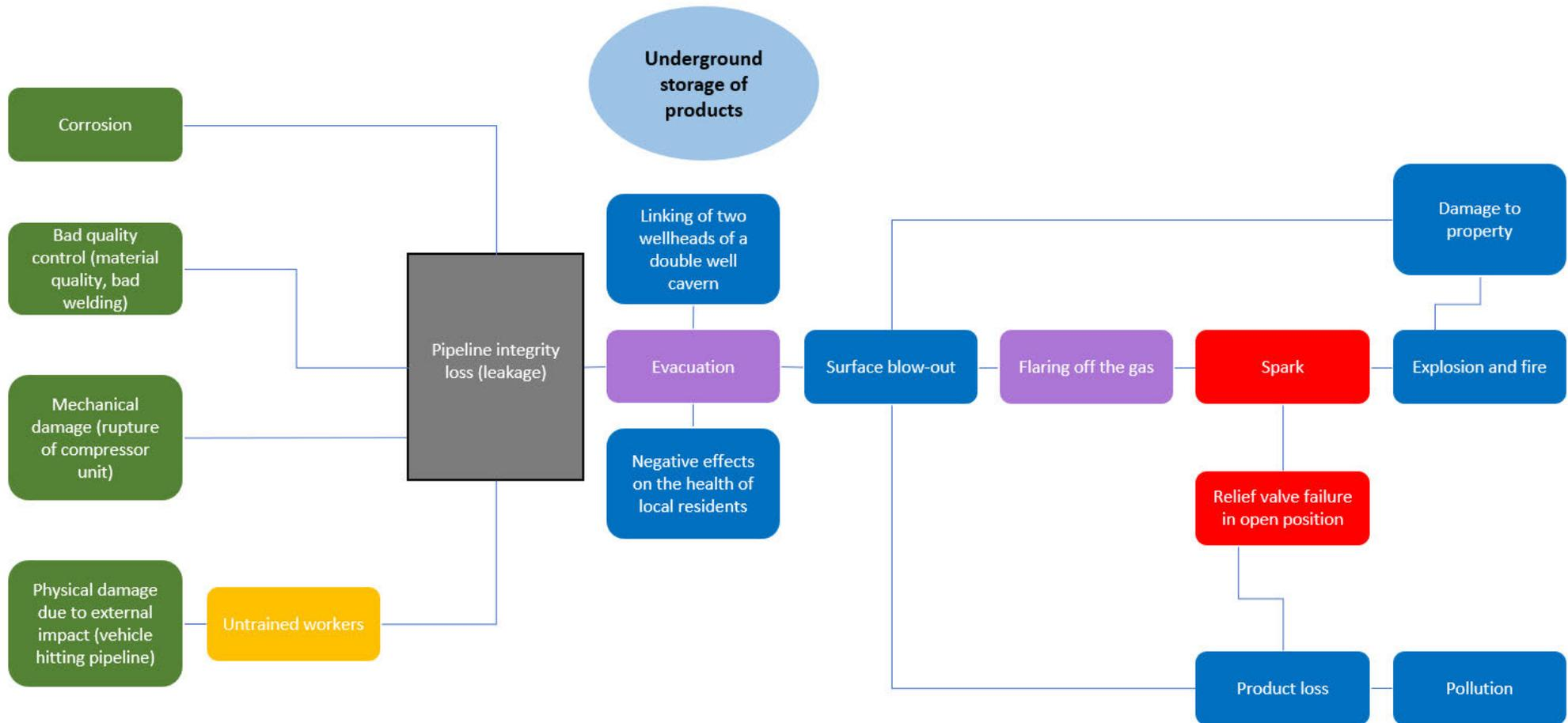
Figure 23 General pipeline integrity loss bow-tie.
