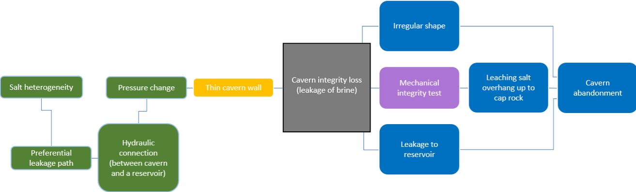
Figure 14 Bow-tie of the Clovelly brine leakage.
