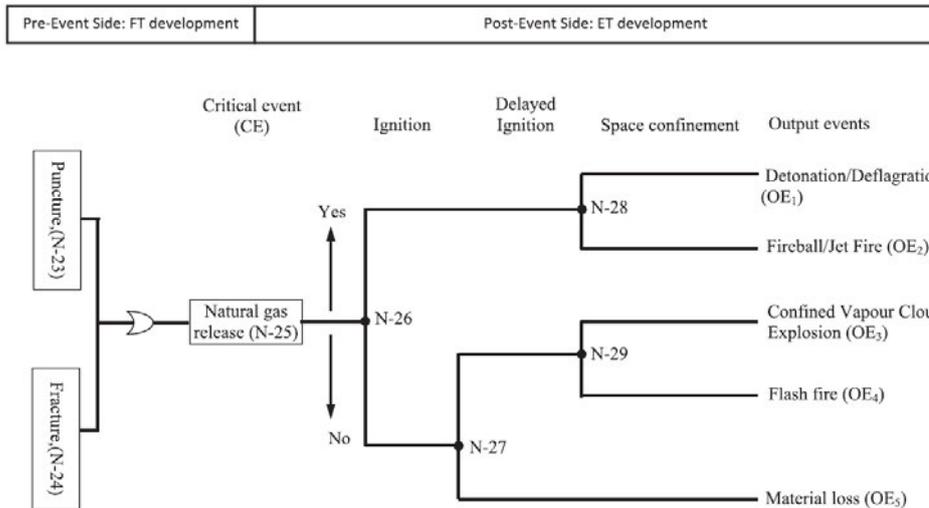
Figure 24 Bow-tie for pipeline integrity loss incidents in gas storage caverns, from Shahriar et al. (2012), who partly modified it from it from Sklavounos & Rigas (2006).
