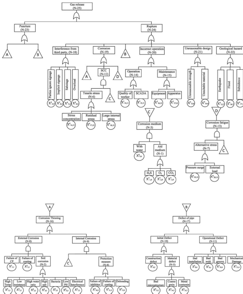
Figure 25 Extensive bow-tie for pipeline integrity loss causes in gas storage caverns, from Shahriar et al. (2012).
