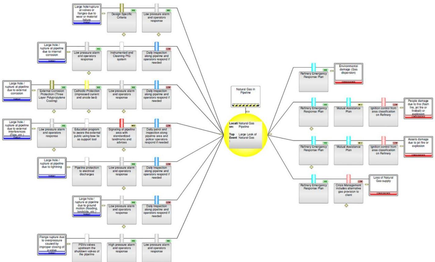
Figure 26 Bow-tie on natural gas pipeline leakages from Muniz et al. (2018).
