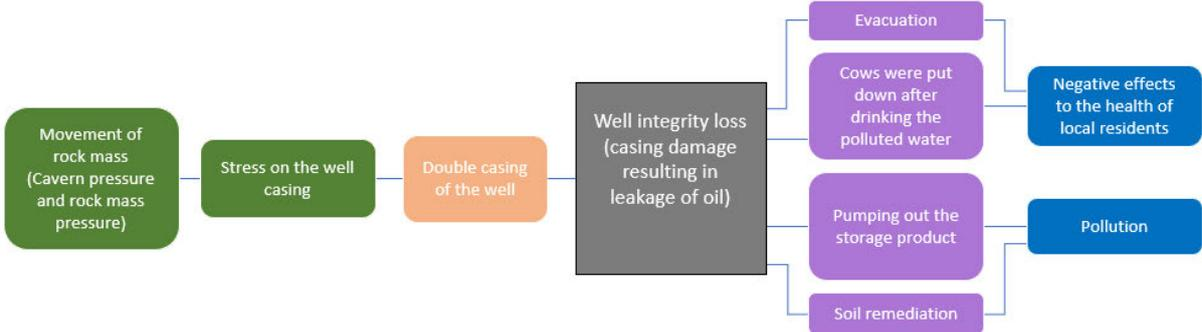
Figure 17 Bow-tie of Epe crude oil spill incident in cavern S5.
