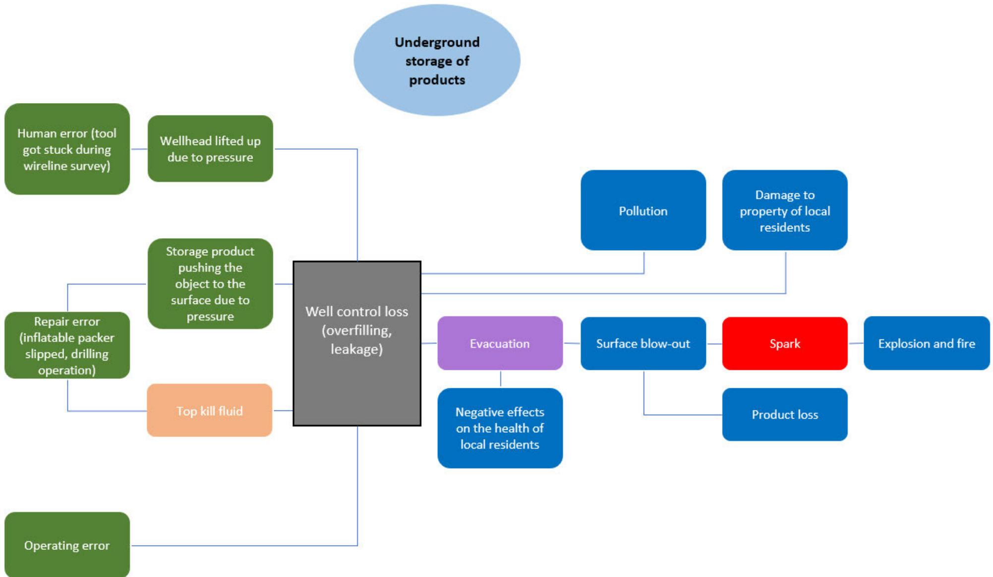
Figure 21 General bow-tie of well control loss incidents.
