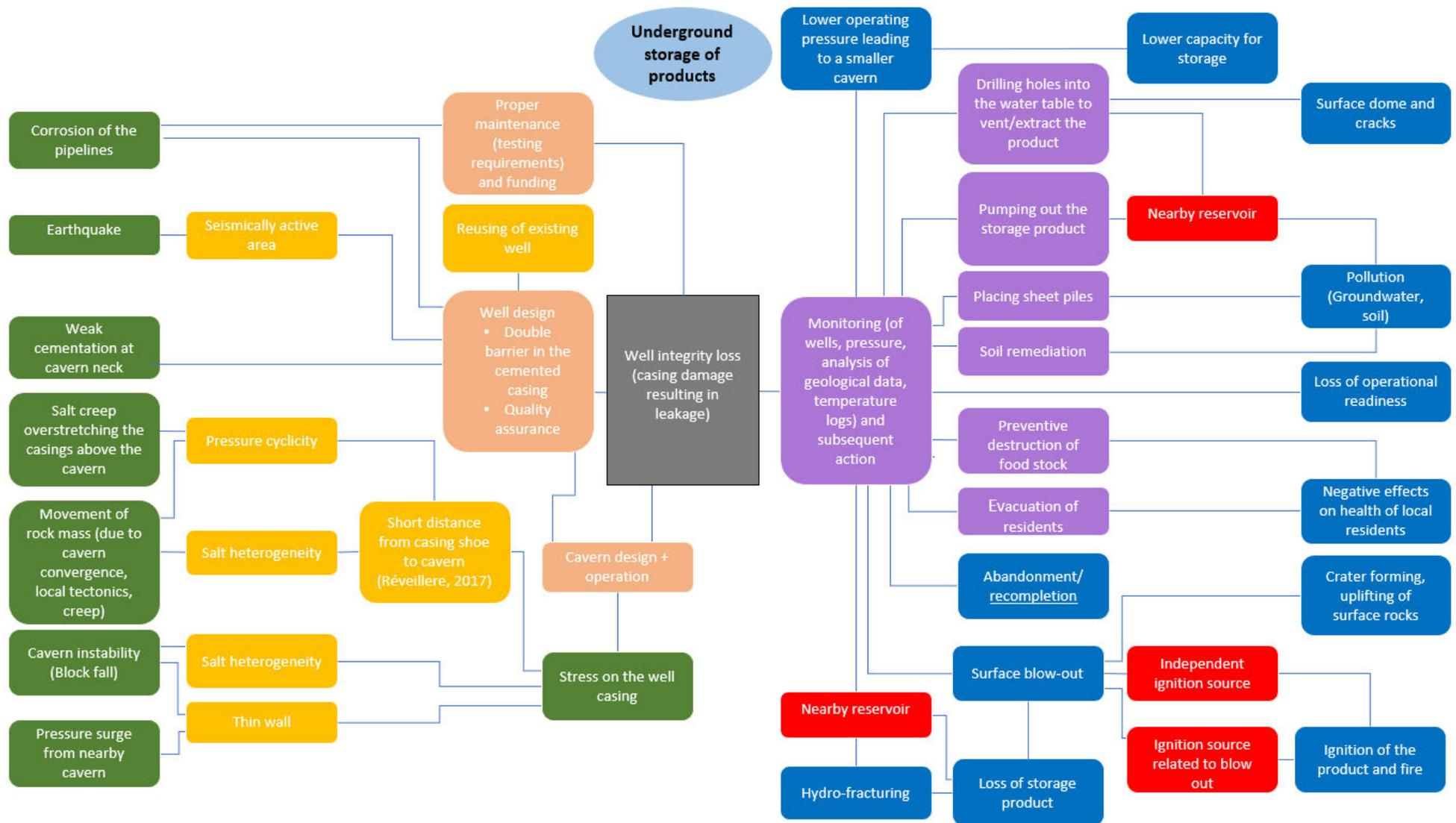
Figure 18 General bow-tie of well integrity loss incidents.
