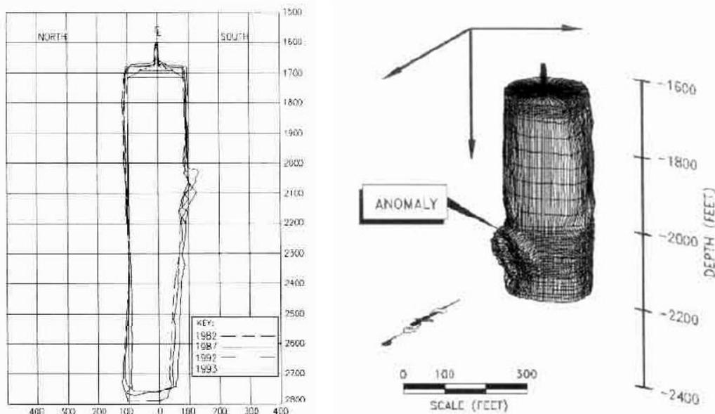
Figure 13 Left: Cavern 14 anomaly growth. Right: sonar survey showing the anomaly bulge. From McCauley et al. (1998).
