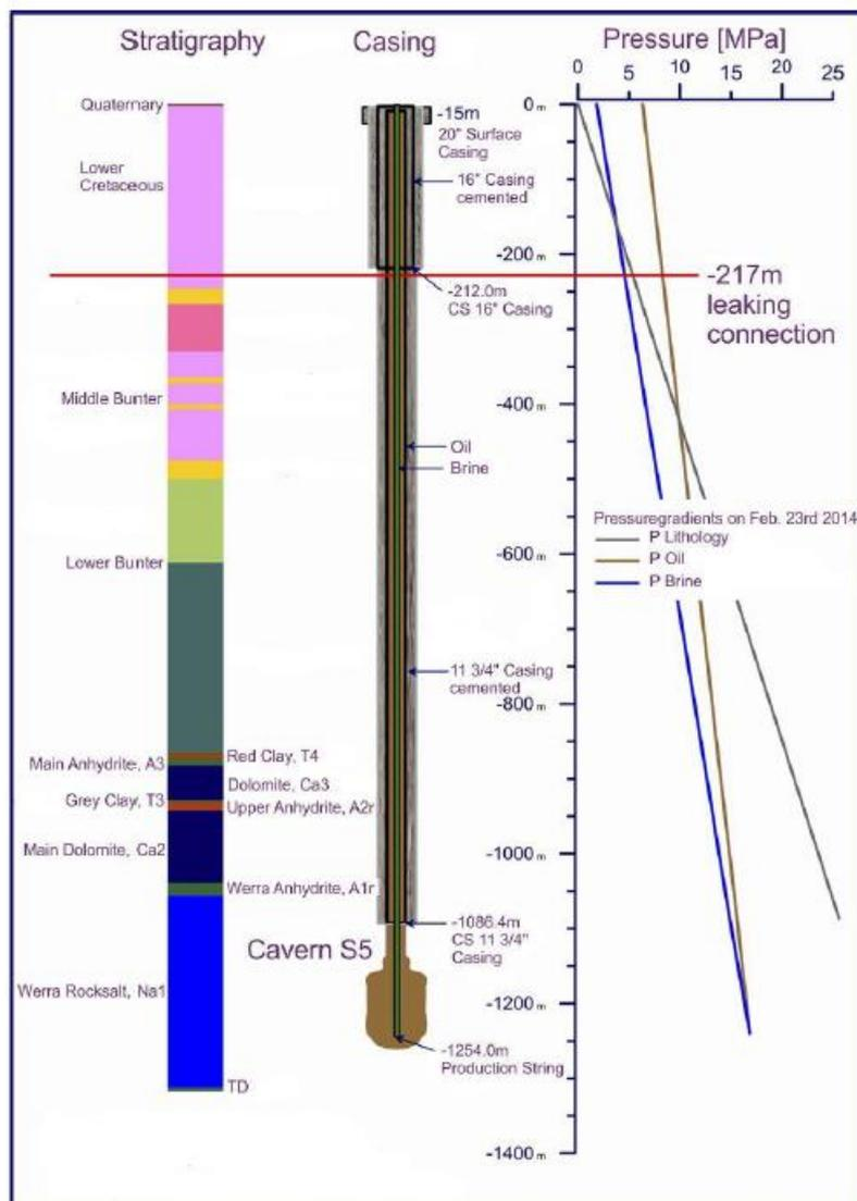
Figure 16 Stratigraphy and pressure of cavern S5 in Epe, Germany. From Hengst (2014).
