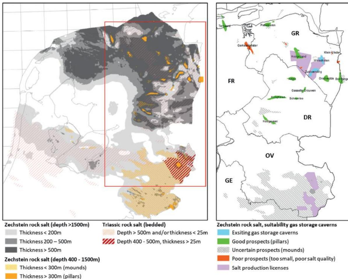
Figure 2 Left: Distribution of the Zechstein and Triassic rock salt. Right: Underground storage and salt production areas, from Juez-Larré et al. (2019).
