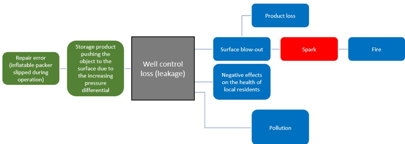
Figure 20 Bow-tie of the West Hackberry well control loss incident.
