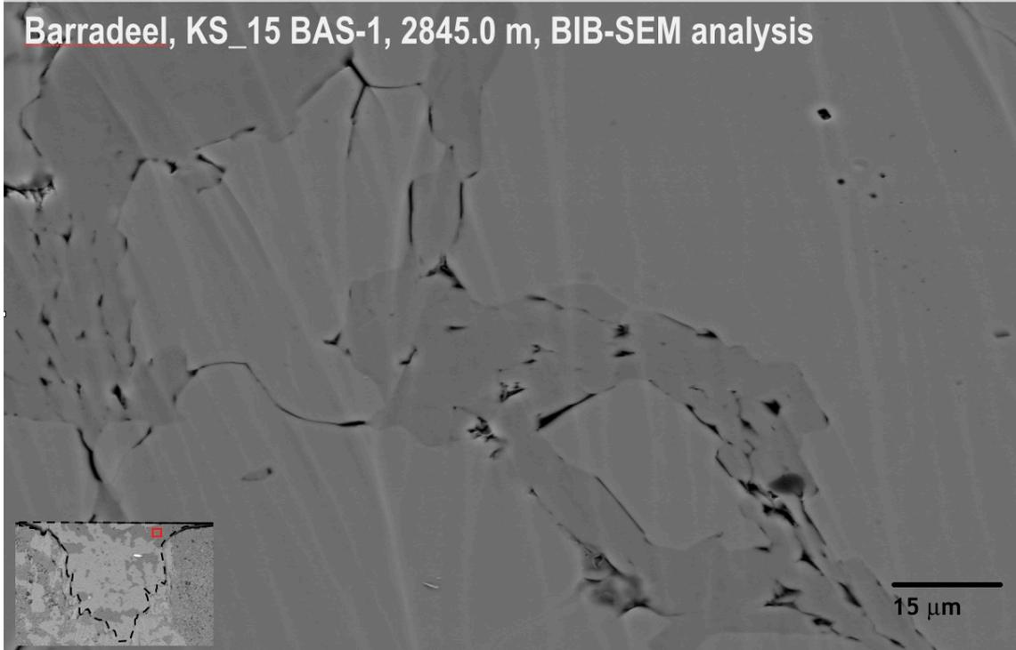
*Figure 71 SEM (BSE) micrograph showing overview on BIB-milled cross section showing porosity in between the three different phases.*
