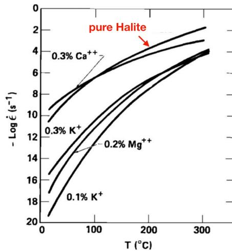
Fig. 13. Expected flow rates in a repository at 880 m depth showing effects of temperature and trace impurities. Based on Eq. (1) and A, Q, and n values summarized in Table 2.
