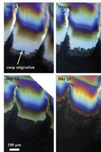
Fig. 5. Micrographs of Crack 2 (see Table 1) showing crack healing in progress: top left, day 4; top right, day 10; bottom left, day 12; bottom right day 20.
