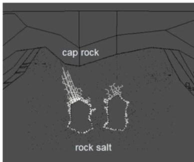
Figure 19. Pressure-driven percolation in brine-filled caverns, 10000 years after sealing of the caverns with reduced percolation threshold along the bedding planes in saliniferous strata (above left cavern S2).
