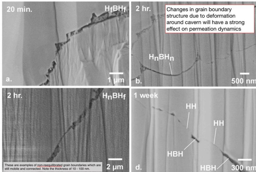
**Figure 28** Cryo-BIB-SEM images of brine-filled grain boundaries in rock salt in various stages of reequilibration. Desbois, G., Urai, J.L., Kukla, P.A., Wollenberg, U., Pérez-Willard, F., Radí, Z., Riholm, S., 2012. Distribution of brine in grain boundaries during static recrystallization in wet, synthetic Halite: Insight from broad ion beam sectioning and SEM observation at cryogenic temperature. *Contributions to Mineralogy and Petrology* 163, 19–31.
