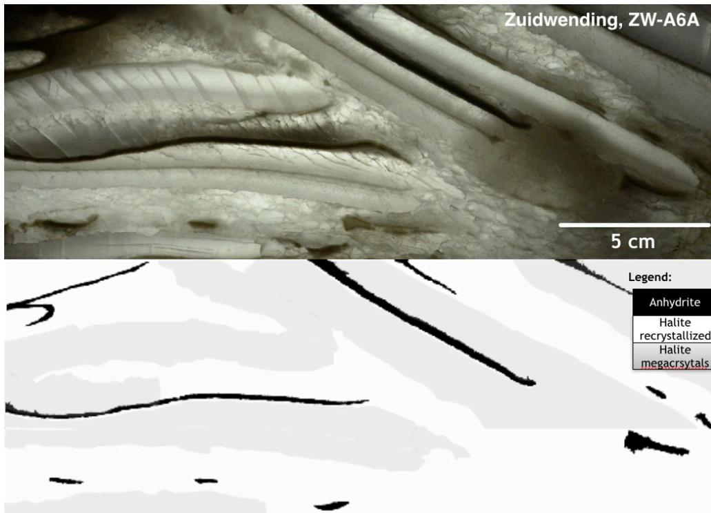
Figure 74 Photographs of slabs using incident and transmitted light (upper picture) were used to estimate areal fractions of the different phase at the scale of the core and to select thin section locations. The slab photos were segmented (lower image) using semi-automated image processing and analysis to derive the area fraction of Anhydrite, recrystallized Halite,
