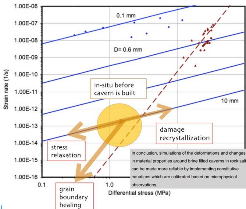
*Figure 42 Based on integration of microphysics and rock mechanics in rock salt geoscience, we now have a reasonably complete set of microphysically based constitutive models which describe the complex rheology of rock salt at low deviatoric stress and low strain rate. Here we propose that integrating this understanding in the salt engineering design will significantly increase the reliability of predictions of the evolution of abandoned caverns.*
