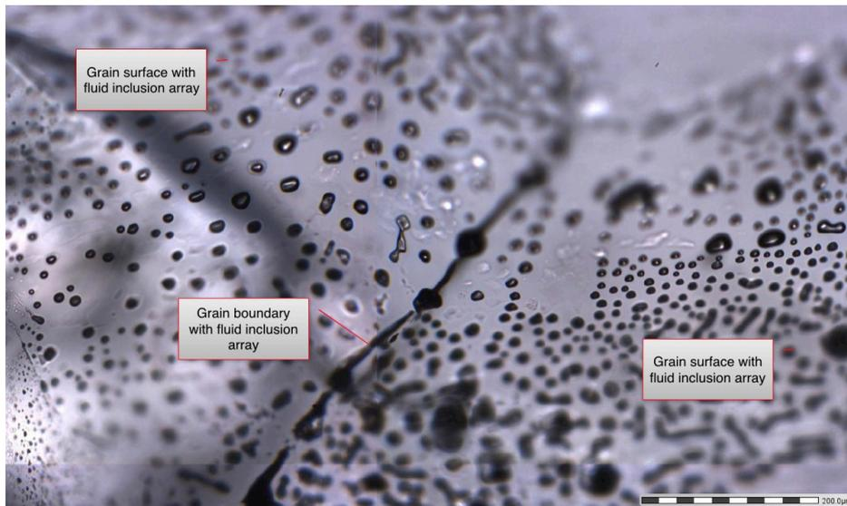
*Figure 77 Zuidwending, KS\_11 ZW-A6A, 599.4 m, grain boundary structure. ViP micrograph showing triple junction of recrystallized Halite grains with fluid inclusion arrays on the grain boundaries.*
