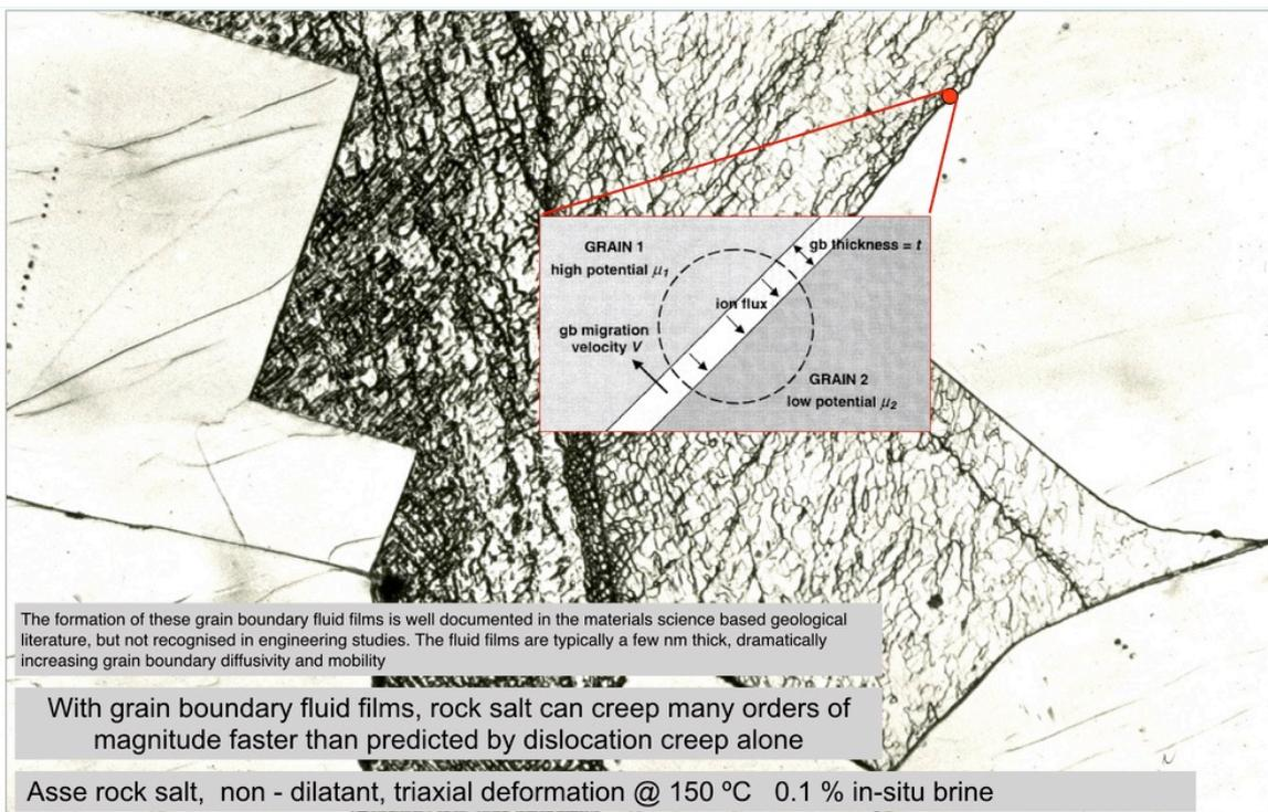
**Figure 23** Fluid filled grain boundaries in rock salt have a dramatically increased mobility and diffusivity, causing major changes in creep and permeation. These microphysical processes must be taken into account for reliable predictions of deformation around salt caverns over long term. After: Urai, J.L., Spiers, C.J., Zwart, H.J., Lister, G.S., 1986. *Weakening of rock salt by water during long-term creep*. Nature 324, 554–557.
