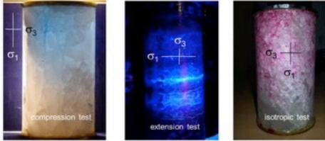
Figure 4: Pressure driven percolation after overcoming the minimum principle stress  $\sigma_3$  directed to the maximum principle stress  $\sigma_1$  within an anisotropic stress field (left and center) and with a homogenous diffusion along all grain boundaries at isotropic stress (right)
