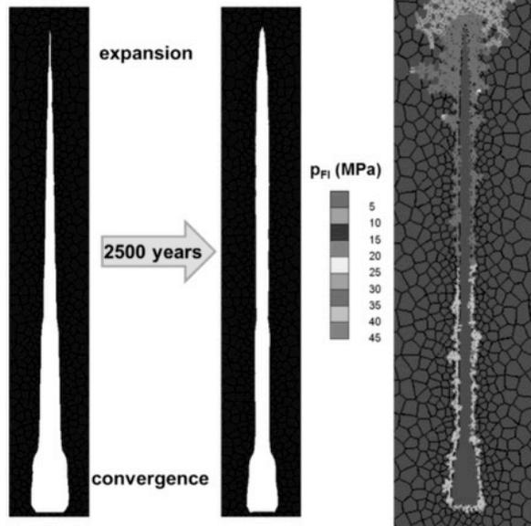
Figure 17. Computed deformation caused by brine pressure, and pressure-driven percolation of a sealed cavern in a depth of 1350–1900 m.
