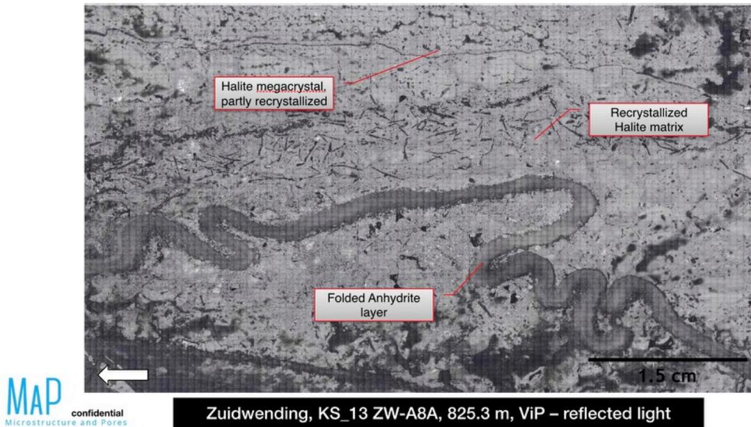
**Figure 78.** *Folded anhydrite layers ViP micrograph acquired in reflected light was used to measure grain- and subgrain size in the recrystallized parts of the thin section. For this purpose, the thin section surface was etched using the protocol proposed by Urai et al. (1987). Image showing overview of the entire cross-section, with folded Anhydrite layers and Halite single crystals embedded into recrystallized Halite matrix.*
