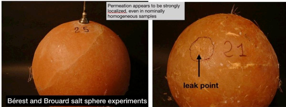
Figure 55 The Paris salt sphere permeation experiments, apparently strongly localized. Bérest, P., Brouard, B., de Greef, V., 1999. Salt permeability testing RFP 98-1 and 2: The influence of permeability and stress on spherical hollow salt samples. Research Report. Laboratoire de Mécanique des Solides (Ecole polytechnique), Paris, France.
