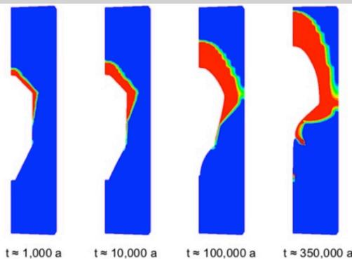
Figure 16. Pressure-driven fluid infiltration processes around a sealed brine-filled cavern
