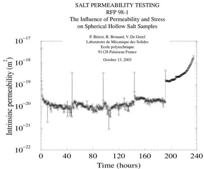
Figure 6: Sphere No. 13 : Permeability increases when cavity pressure is larger than overburden pressure. The increase is significant when the cavity pressure is larger than the overburden pressure by 1.3 MPa (i.e., the last pressure step).
