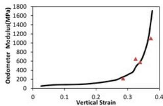
Fig. 4. Calibration of the elastic properties (solid line: experimental results; red dots: calibrated model)
