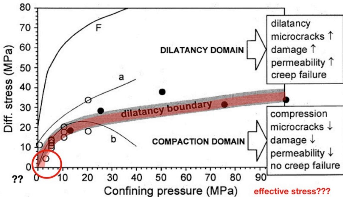
Figure 19 The classic study on the dilatancy boundary in rock salt. Non-dilatant deformation is often used as a criterion for integrity in salt engineering. After: Popp, T., Kern, H., 2000. Monitoring the state of micro fracturing in rock salt during deformation by combined measurements of permeability and P- and S- wave velocities. Physics and Chemistry of the Earth, Part A: Solid Earth and Geodesy 25, 149–154.
