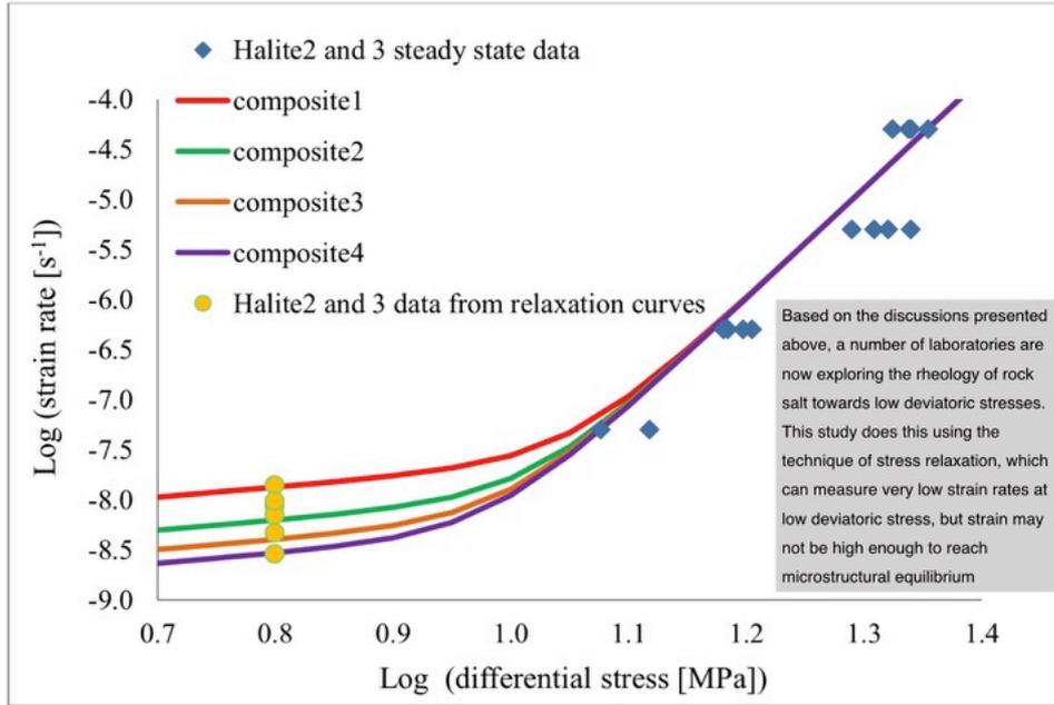
Figure 37 Based on the discussions presented above, a number of laboratories are now exploring the rheology of rock salt towards low deviatoric stresses. This study does this using the technique of stress relaxation, which can measure very low strain rates at low deviatoric stress, but strain may not be high enough to reach microstructural equilibrium. After: Muhammad, N., 2014. Deformation and transport processes in salt rocks; PhD Thesis, Utrecht University.
