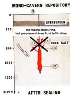
Figure 3. Abandoned and sealed liquid-filled salt cavity (Lux 2009)
