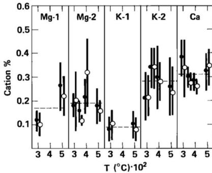
Fig. 1. Microprobe analyses showing dopant concentrations in deformed samples. The dashed horizontal line represents the average concentration. Core and rim compositions of single crystals are denoted by solid and open circles, respectively.
