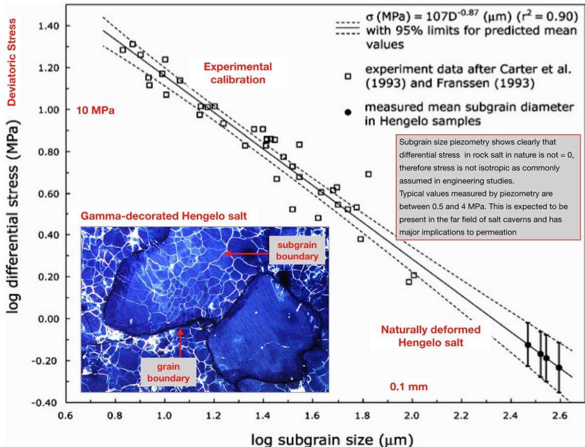
**Figure 10** Subgrain size piezometry using Gamma-decoration of microstructure in rock salt from a core from the Hengelo cavern field, the Netherlands. After: Schleder, Z., Urai, J.L., 2005. Microstructural evolution of deformation- modified primary Halite from Hengelo, the Netherlands. *International Journal of Earth Sciences* 94, 941–956.
