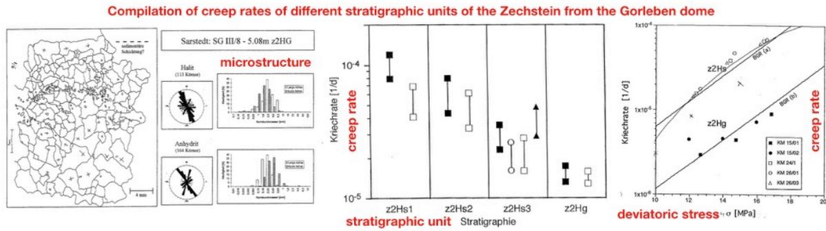
Figure 18 An interesting attempt to correlate creep properties of rock salt samples from different stratigraphic units based on Microstructure (grain size and inclusions). After: Popp, T., 1994. Gefügekundliche Untersuchungen an Salzgestein der Staffurt-Folge aus dem Salzstock Sarstedt. Research Report No. 112624. BGR, Hannover, Germany.
