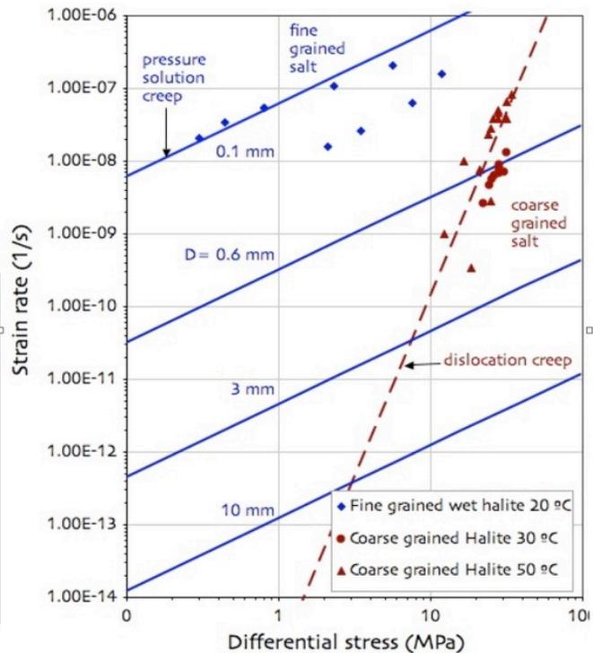
**Figure 22** This is a summary of the main microphysical deformation mechanisms in rock salt. They can all operate simultaneously depending on micro fabric and physical conditions, and they are associated with very different mechanical and transport properties. After: Urai, J.L., Schleder, Z., Spiers, C.J., Kukla, P.A., 2008. *Flow and Transport Properties of Salt Rocks. Dynamics of Complex Intracontinental Basins: The Central European Basin System*. Springer, 277–290.
