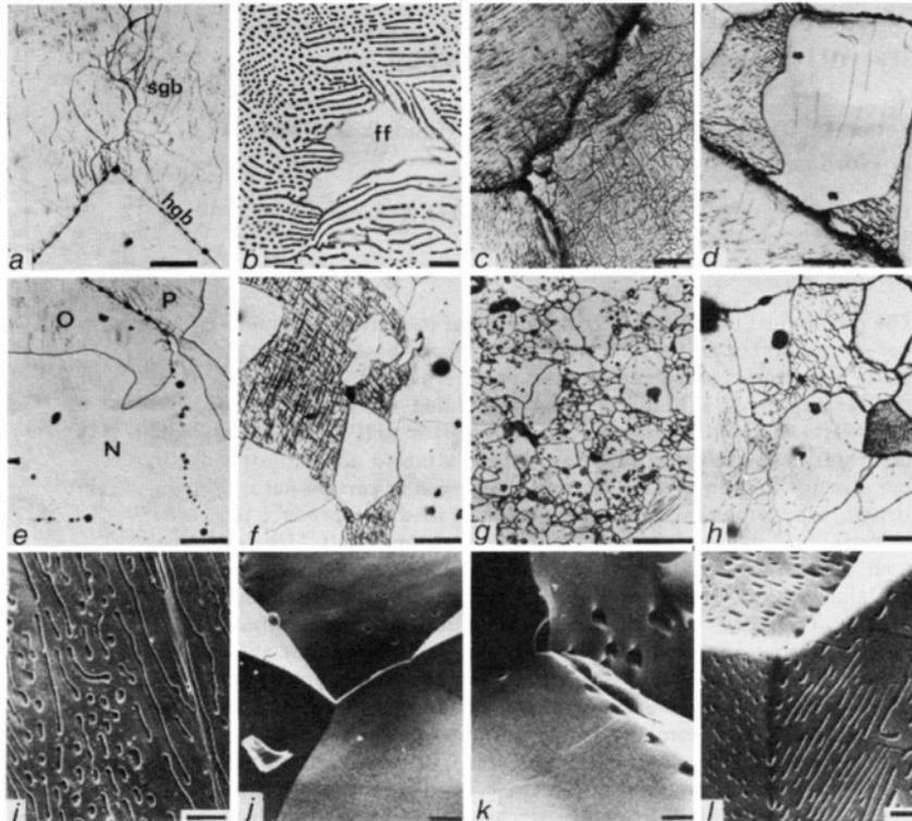
Asse Speisesalz: small amount of inherent brine inclusions lead to rapid grain boundary migration and pressure solution
