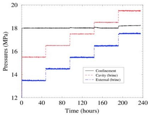
If cavity pressure becomes 1 MPa higher than the minimum stress, permeability starts to increase rapidly
