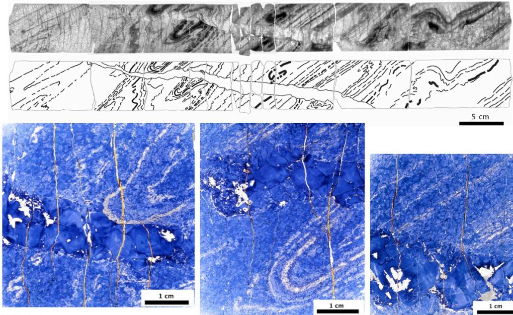
Figure 59. Natural example of hydrofracturing in rock salt, followed by healing of the fracture. After: Schleder, Z., Urai, J.L., Nollet, S., Hilgers, C., 2008. Solution-precipitation creep and fluid flow in Halite: A case study of Zechstein (Z1) rocksalt from Neuhoof salt mine (Germany). *International Journal of Earth Sciences* 97, 1045–1056.
