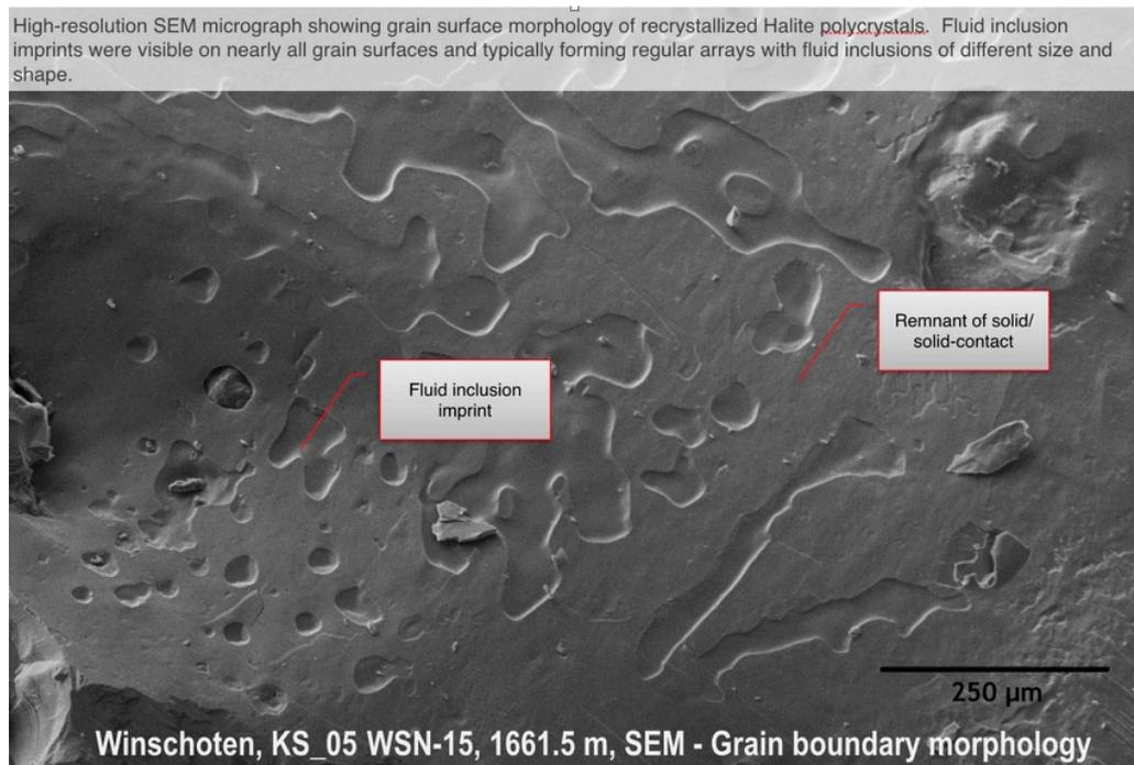
*Figure 80. Typical grain boundary structure in the recrystallized part of the Winschoten core. In this SEM SEII image, the image is of a grain's surface after it was separated from another grain along a grain boundary.*
